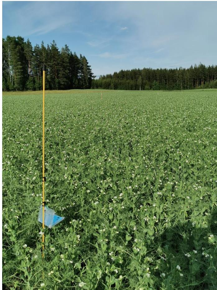
3. The Trapview Standard Delta: Wind sensitive (big and light), opens easily by itself and material wilts and softens (duration 1 growing season ?). - Taping demanded! Fastening threads weak > own systems...
